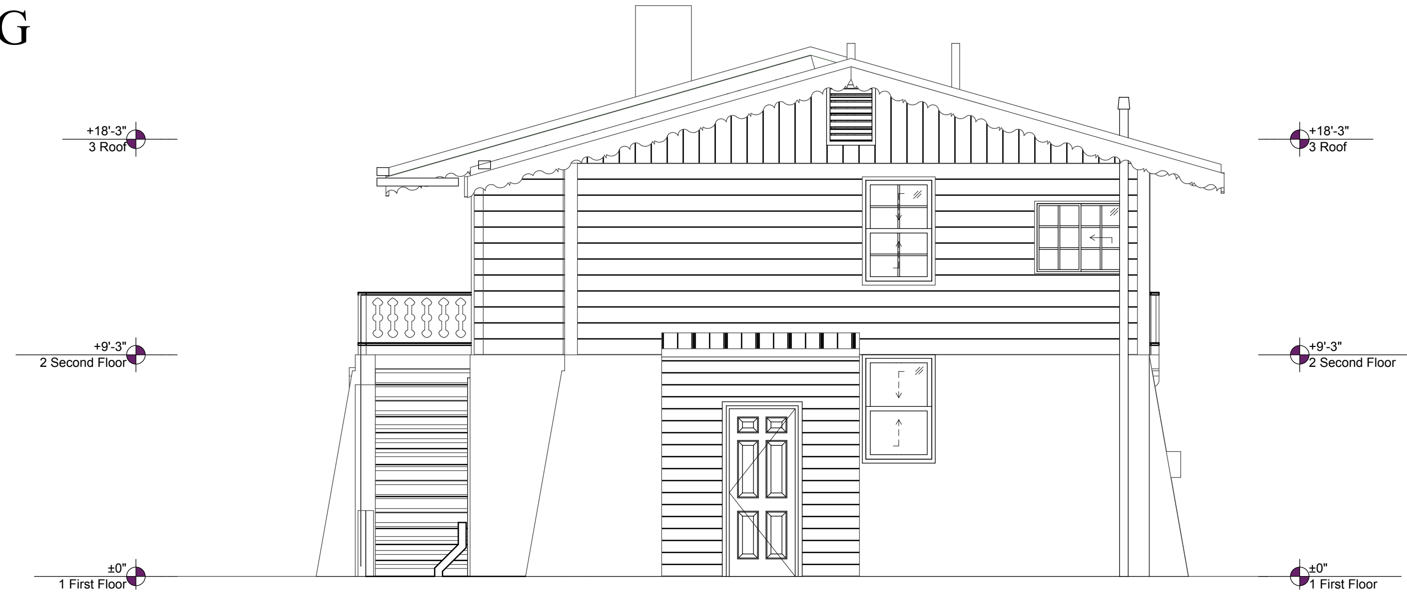
1 H3 Existing North Elevation SCALE: 1/4" = 1'-0"
