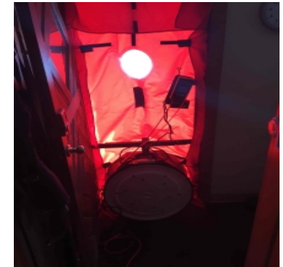
Blower door set up for the pressure test.
